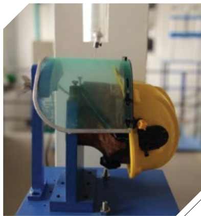
PENETRATION RESISTANCE TEST
