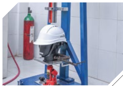
PENETRATION RESISTANCE TEST
