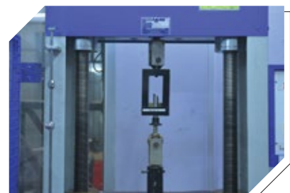
STATIC TEST OF TYPE B ANCHOR
