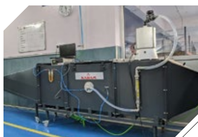
DOLOMITE DUST CLOGGING TEST
